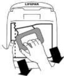
Hold down the left side of the electrode packet with one hand and pull the red packet handle down with the other.
